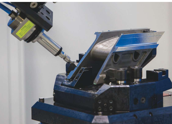
A robot polishes a nozzle for a gas turbine. (Source: GE Oil & Gas)
