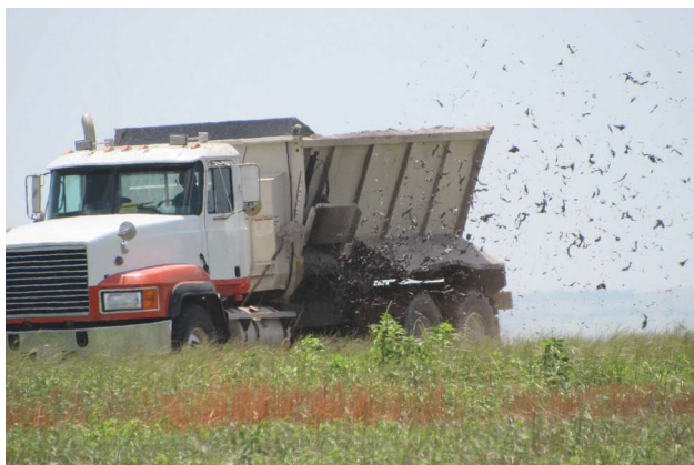
A land farmer distributes drilling waste over agricultural land. Drilling waste can include chlorides, heavy metals, hydrocarbons and other chemicals and additives that are necessary for drilling a well. (Source: Scott Environmental Services)
