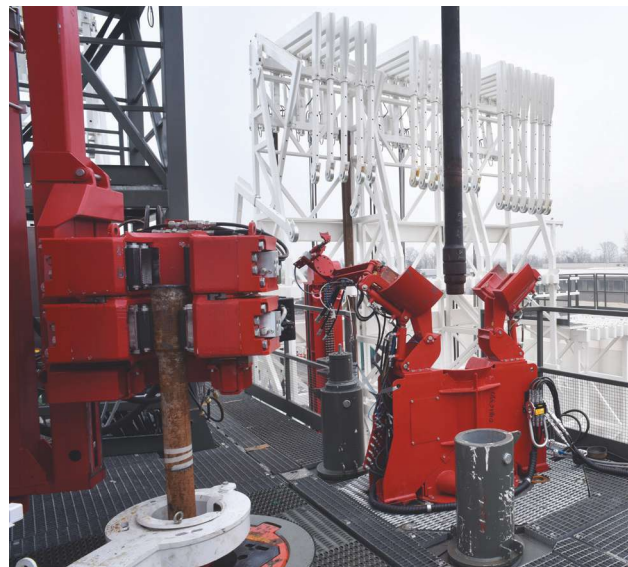
The HH-300 hydraulic hoist 600,000-lb hookload capacity drilling rig has been performing operations with DATS for the past year. (Source: Drillmec)
