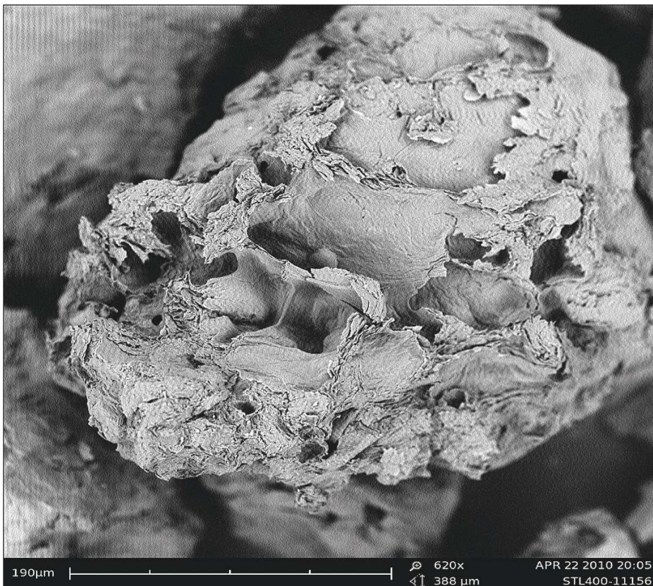
FIGURE 1. The STEELSEAL's irregular shape and open pores lock particles in place. (Source: Halliburton)
