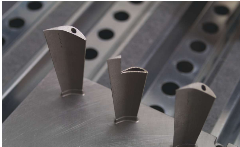
The 3-D-printed turbine blades are manufactured at the Talamona plant. (Source: GE Oil & Gas)
