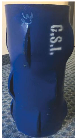
Perforations made by the hydromechanical tool can be indexed in-hole in a spiral effect for improved fluid sweep. (Source: Energy Fishing and Rental Inc.)
