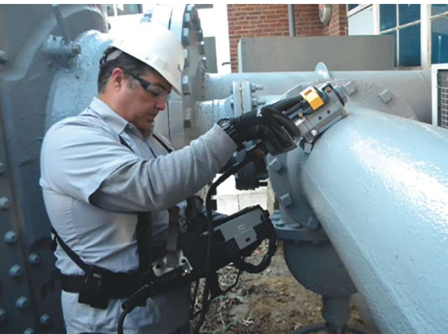
Instant C-scan images of weld defects, corrosion and various other defects are available with the AcoustoCam i700. (Source: PRNewsFoto/Imperium Inc.)
