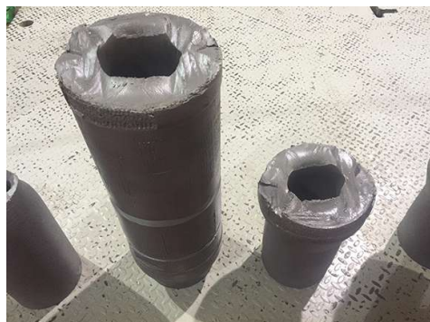
Tool joint hardbanding is sheared off-center by the Cameron BroadShear technology ram. (Source: Schlumberger)
