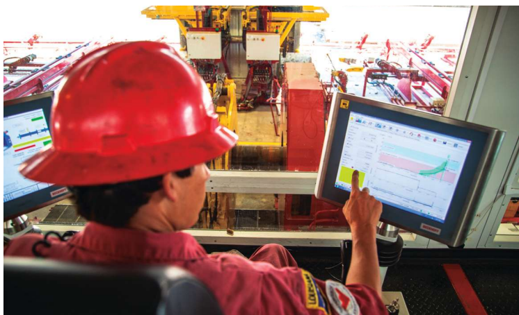
A technician monitors and evaluates whether or not each connection is secure and ready to be run into the wellbore. (Source: Weatherford)
