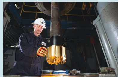
Talon Force bits with 1-in. Stabilis cutters have improved ROP and drilling efficiency for operators worldwide. (Source: Baker Hughes)
