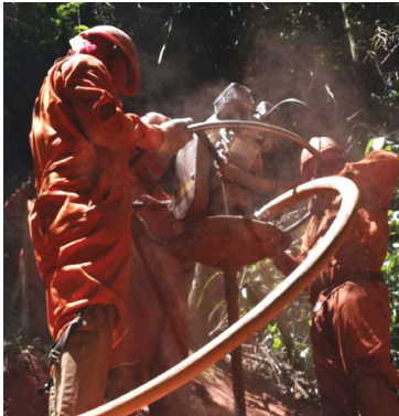
FIGURE 1. SAE shot a 3-D survey in 2014 in Bolivia for Repsol involving 27,000 wireless stations and high-sensitivity single-sensors. This photo shows the efforts made by the seismic crew to place sources and receivers. (Source: Geospace Technologies)
