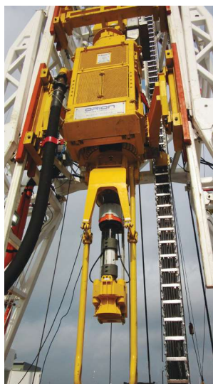
GE's Equipment Insight will help GDS International improve its data collection, analytics and management capabilities in equipment such as the pictured GDM500 top drive system in an Orion Drilling mast. (Source: GE)
