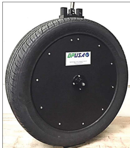
The MV-24 uses opposed piston transducers run by a 6.3-hp motor that can drive the transducer from 0 Hz to 100 Hz at sweep rates from 3 sec to 30 sec in length. (Source: GPUSA)
