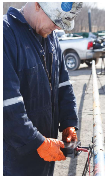
A PNP gun string is surface-tested prior to connecting the cable head. (Source: DynaEnergetics)
