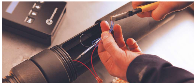
A worker wires a DynaSelect intrinsically safe integrated switch detonator into a perforating gun. (Source: DynaEnergetics)
