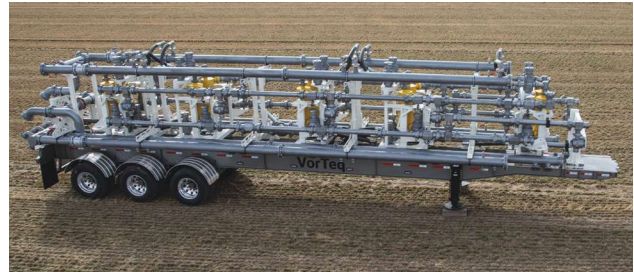
A new missile developed by Energy Recovery could cut the cost of hydraulic fracturing by an estimated $4 to $5 per barrel. Liberty Oil-field Services conducted a field test of the VorTeq missile in December 2015. (Source: Energy Recovery)
