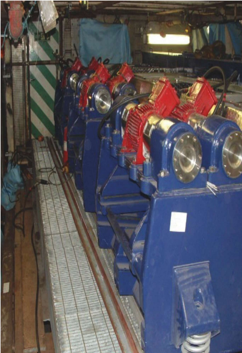
An additional mud pump was added on three out of four platforms. Apache converted from the use of water-based mud to OBM for improved hole stability.
