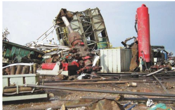
The BOP stack in the center of the photo leans to the left after the EF5 tornado struck the rig. The rotary table is on the top of the mud pit to the left of the BOP. All rig hands survived. (Source: Cactus Drilling)
