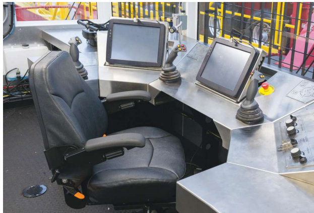
Operator control rooms on the T500XD and T250XD are equipped with joysticks and large touchscreens that allow rapid navigation to all operational and diagnostic data from the rig. This makes real-time data from any sensor in the system literally at a user's fingertips. With an active internet connection, the live data can be transmitted to any connected offsite location. (Source: Schramm)
