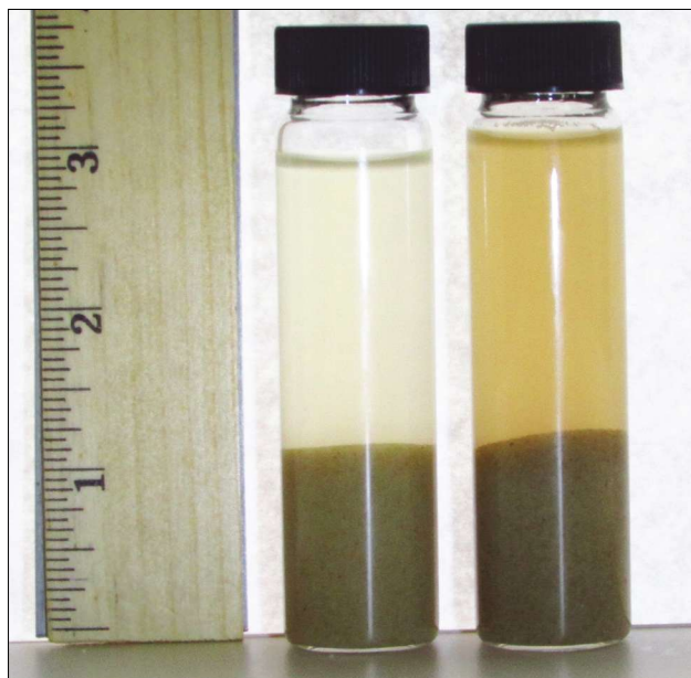
FIGURE 2. Shown are samples of SandGuard (left) and uncoated sand (right) after settling out for 30 seconds. (Source: Superior Silica Sands)
