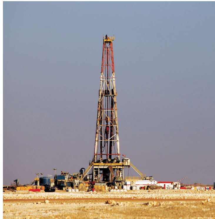
The LR5 rig is on one of the world's largest unconventional gas resources, the Khazzan Field in Block 61 onshore Oman, where operator BP will drill horizontal wells and use hydraulic fracturing to stimulate production from the tight gas reservoir. (Source: BP)
