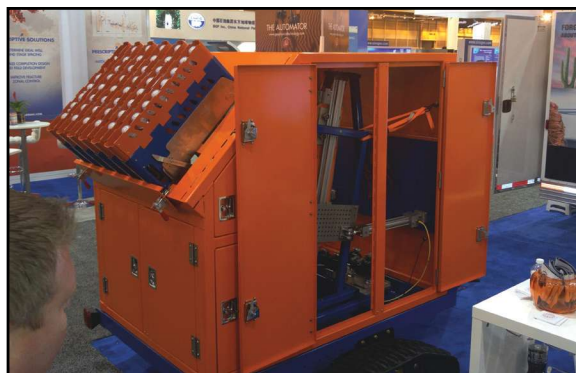
The Automator is designed to plant geophones robotically, saving time and money in land and transition zone seismic acquisition. (Source: GTI)
