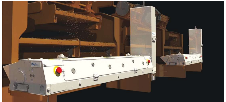
FIGURE 1. The CLEAR hole cleaning and wellbore risk reduction service incorporates a cuttings flowmeter at the end of each shale shaker. The flowmeter catches and weighs cuttings as they fall off the screen but without obscuring access to the shaker. (Source: Schlumberger)
