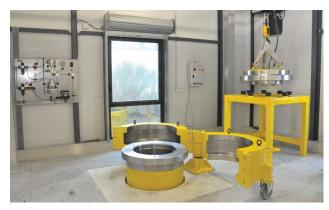
A MacArtney hydrostatic pressure vessel has been installed within a new test environment. (Source: MacArtney)
