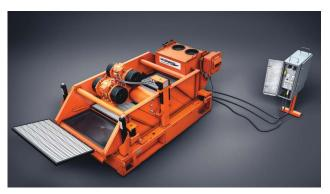
The SCREEN PULSE separator recovers drilling fluid and can generate a drier cuttings discharge from the shale shaker. (Source: Schlumberger)
