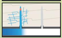
Additional fracturing fluid and proppant are then pumped and redirected to the smaller fracture systems to create a more complex fracture.
