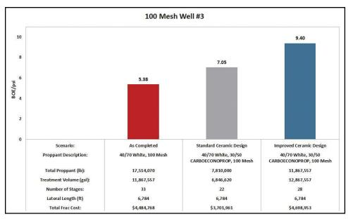
The chart shows the predicted impact of alternative completion and frack designs on Operator C's underperforming, all-white sand well. (Source: Carbo Ceramics)
