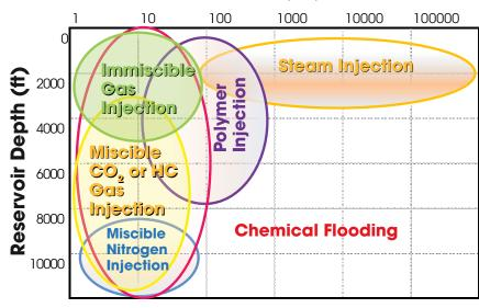
FIGURE 1. This figure shows the typical range of EOR technology applications. (Source: Repsol)
