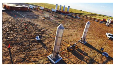
A closed-loop tank ventilation and combustion system replaces conventional methods of flaring excess methane and vapors on hydraulic fracturing sites. (Source: Select Energy Services)
