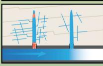
Fluid and proppant are redirected to another perforation set that was not previously accepting any fluid, and a new fracture is created.
