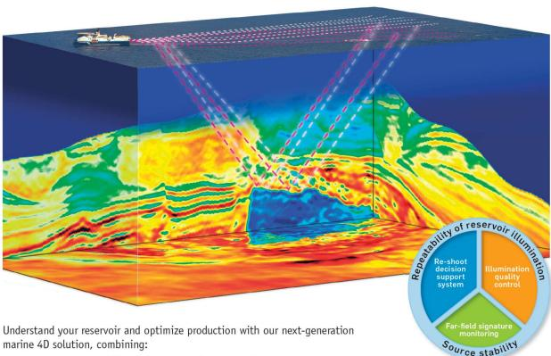
Precise 4D repeatability from powerful integrated source, streamer and vessel steering
