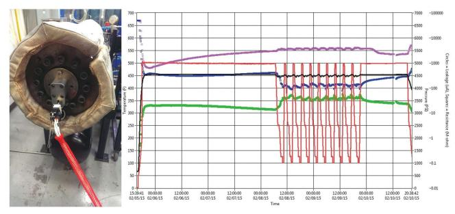
FIGURE 2. The *in situ* chamber penetration and parametric overlay plot shows the electrical feed-through on the environmental autoclave and the electrical performance at temperature as the connecter underwent pressure cycling. (Source: ITT Corp.)
