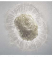
Propel SSP proppant transport technology swells upon contact with water to go farther and higher into the formation, expanding the reservoir drainage radius from a longer effective fracture half-length.
