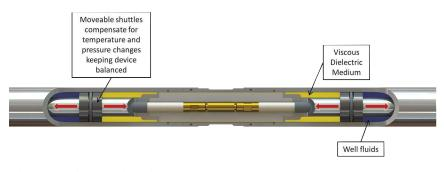
FIGURE 1. Key features of k-PaC Technology's pressure-balancing concept are the movable barriers that encapsulate a viscous dielectric medium that can accommodate well pressure without creating a large pressure differential across the connector. (Source: ITT Corp.)
