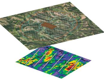
Global's innovative seismic acquisition and quick delivery of 3D and ambient seismic attributes provides detailed and actionable information for well planning and completion design.
