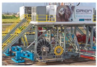
The IDS ReelRig power and communication cable spooling skid is shown attached to the substructure of Orion Drilling's new Aries Rig #18. (Source: Integrated Drive Systems)
