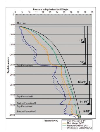
A typical deepwater subsurface pressure profile exemplifies the challenges of tight-tolerance casing design. (Source: Weatherford)
