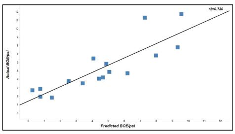
The ANN model compares predicted boe/psi vs. actual boe/psi for Operator C of Eagle Ford Shale wells (validation data). (Source: Carbo Ceramics)
