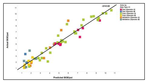
The ANN model compares predicted boe/psi vs. actual boe/psi for operators A and B of Eagle Ford Shale wells (train, test and validation data). (Source: Carbo Ceramics)
