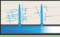
With time, temperature, and an aqueous- or oil-based carrier fluid, the diverter will dissolve, leaving a more conductive fracture geometry. ond was a phenomenon known as imparted stress shadowing. This phenomenon occurs when two hydraulic fractures are placed adjacent to one another and the presence of one frack impacts the stress experienced by the other.
