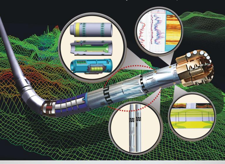
The GW-NB system consists of measurement transmission motors, a wireless receiving system, a positive pulse of wireless LWD system, and surface processors and geosteering decision software. It is designed to improve the discovery rate for exploratory wells, drilling encounter rates and oil recovery for development wells.
