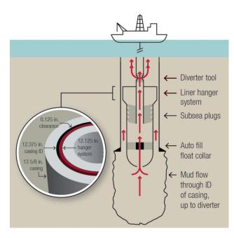
Surge management and tight tolerance are realized by running a diverter tool in conjunction with auto-fill float equipment to divert displaced fluids from the casing running string into the annulus. (Source: Weatherford)
