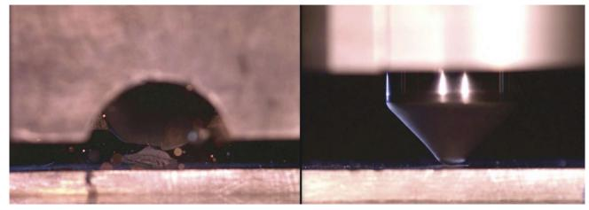
FIGURE 2. A comparison shows a Stinger element (right) vs. a conventional PDC cutter (left) after impacting a hardened steel block at 18,000 lbf to simulate drilling into a hard limestone at 60 ft/hr. (Source: Schlumberger)
