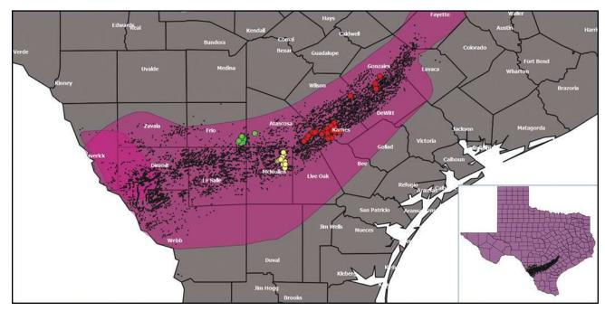
The locations of the wells used in this study (red, Operator A; green, Operator B; and yellow, Operator C), are compared to those of other wells drilled since 2008 (black dots). (Source: Carbo Ceramics)
