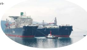
Allseas' Pioneering Spirit heavy lift vessel will first remove Brent Delta's topsides, which weigh 24,000 tonnes and will be lifted in approximately 10 seconds, said Shell. (Source: Allseas)
