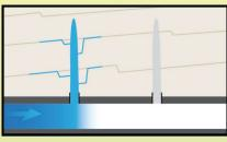
First, a portion of the scheduled fracturing fluid and proppant is pumped, creating a fracture with minimal complexity.
