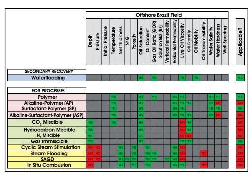
FIGURE 2. EOR case study pre-screening results indicate that polymers provide the best and most costeffective recovery for this particular field. (Source: Repsol)
