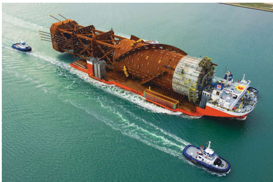
The Technip-built hull for Anadarko Petroleum’s deepwater Lucius spar is seen being transported by Dockwise’s Mighty Servant 1 barge. Lucius was due onstream before the end of 2014, with the operator opting for a ‘design one, build two’ approach that saw it repeat the process for its Heidelberg development, also in the GoM. This saw Anadarko apply lessons from the first project, which it says has resulted in significant cost savings and a shortening of the development cycle by up to 18 months. Heidelberg is due onstream mid-2016. (Source: Dockwise)
