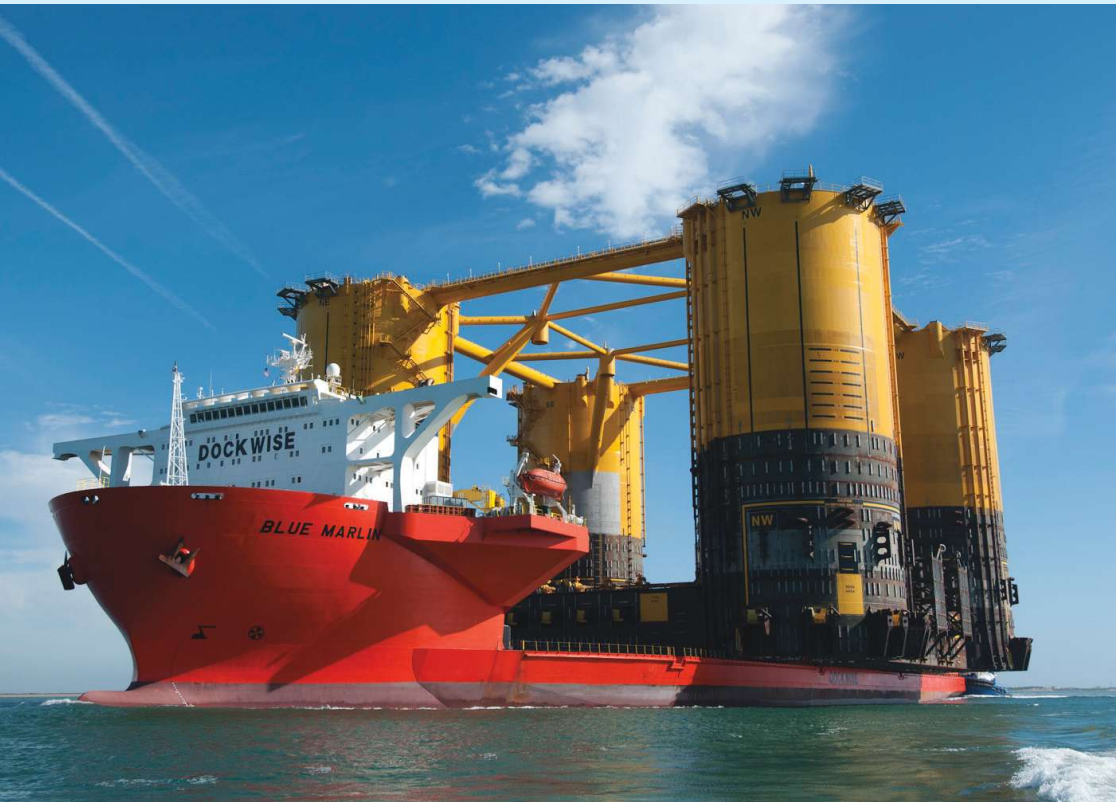
LEFT: Dockwise transported the Olympus hull from Busan, Korea, to Ingleside, Texas, onboard the Blue Marlin . CENTER: The direct vertical access rig module was installed at Kiewit Offshore Services yard in Ingleside, Texas. RIGHT: The accommodations module is lowered onto the deck of the Olympus TLP. (Source: Shell)
