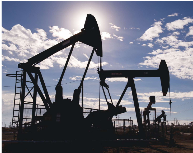
SRPs are the most common method for shale oil in deep deviated wells, so the industry is addressing challenges such as the MTBF caused by side-loading and misalignment of the pumpjack.
