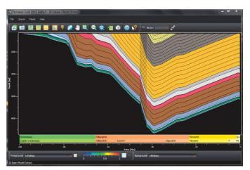
FIGURE 3. This image shows the burial history from the basin model. (Source: Landmark)
