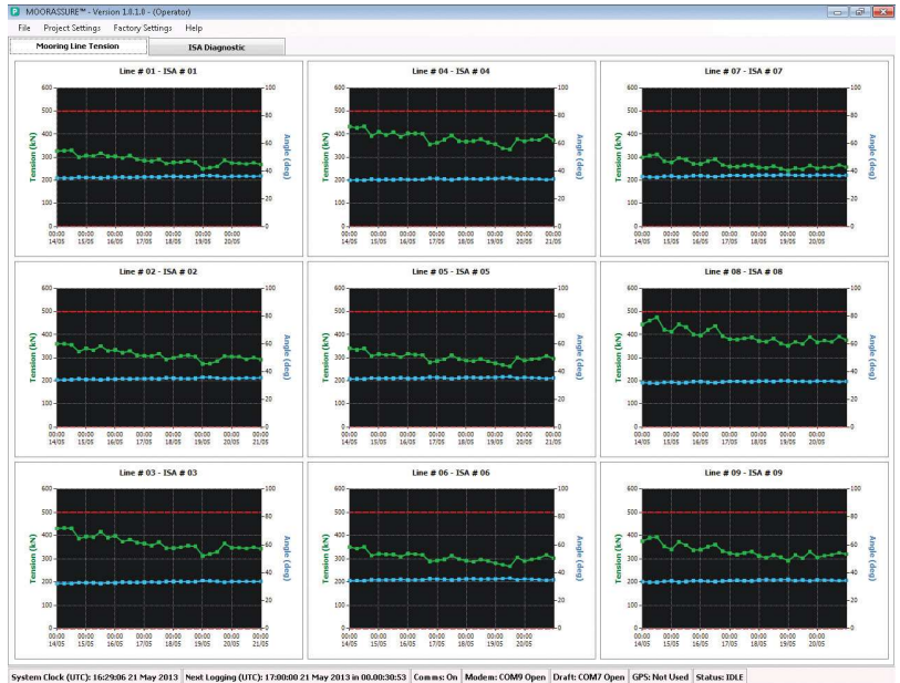
FIGURE 3. This MoorASSURE software screenshot shows an example of the angle and tension readings on each mooring line. (Source: Pulse Structural Monitoring)
