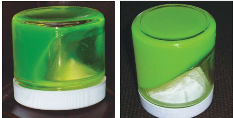
The image on the left shows an SPI gel with internal initiator. The image on the right shows an SPI gel with CO 2 initiator. (Source: National Energy Technology Laboratory)
