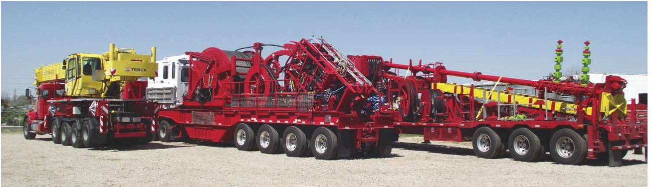
FIGURE 2. The new CT package includes a 60-ton crane. (Source: Boots & Coots, a Halliburton company)
