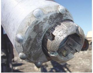
Ways to improve drilling efficiency are a continuous area of focus around the world. DURA Drilling's high-speed dual-drilling string technology (featuring both an inner and an outer drill-string) was showcased to Middle Eastern ITF members as they look to collaborate on technology that will help enhance the region's reservoir recovery rates. (Source: Dura Drilling)
