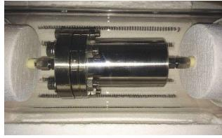
A thermal desorption chamber is used to induce desorption of mercury from steel test coupons cut from hydrocarbon process systems. (Source: PEI)
