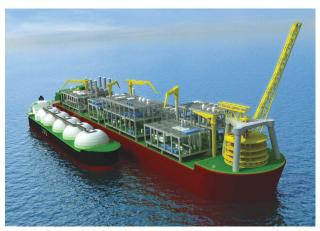
FMC Technologies' OLAF system, another Spotlight Award winner, will be used on Shell's giant *Prelude* FLNG vessel to offload LNG to carriers. (Source: Shell)
