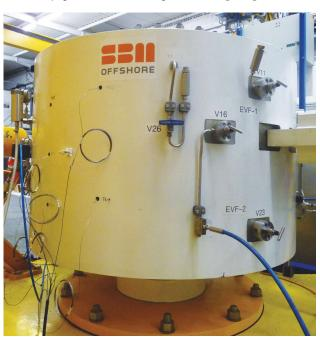
SBM Offshore's VHP Fluid Swivel was one of the Spotlight Award winners at OTC, with the technology enabling the use of FPSO vessels for the development of ultrahigh pressure reservoirs and being qualified to handle pressures of up to 12,000 psi. (Source: SBM Offshore)
