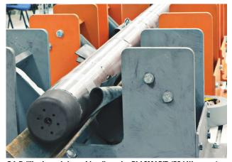
GA Drilling's prototype 4-in. diameter PLASMABIT (50-kW power) drilling system generated high levels of interest at the ITF's event in Abu Dhabi. The system is part of a JIP and is based on using focused electric plasma energy. The first applications of this technology are likely to be in operations where steel removal is necessary such as plugging and abandonment. (Source: GA Drilling)
