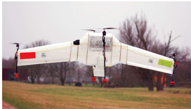
FIGURE 4. A hovering ATMOV prepares to plant a calibration sensor. When flying longer distances, the wing is rotated 90 degrees, allowing high speeds. (Source: Delft University of Technology)
