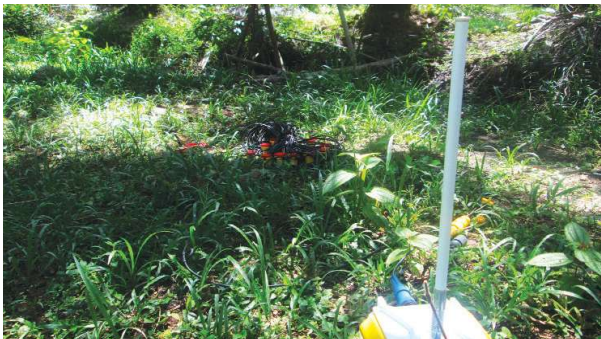
In Ohio, horizontal drilling within 4.8 km of a known fault or area of seismic activity would require companies to install seismic monitors such as these. (Source: Wireless Seismic)
