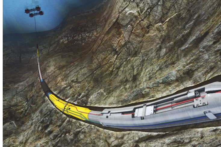
Fiber-optic sensors enable distributed temperature, pressure and acoustic sensing downhole. (Source: Baker Hughes)
