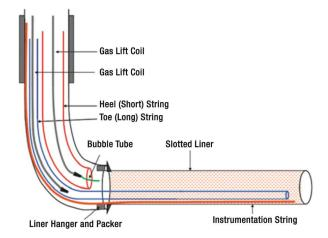
FIGURE 1. This represents an example of a dual-tubing well configuration. (Images courtesy of Energy Resources Conservation Board Alberta)
