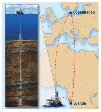
During the well test, real-time downhole data was wirelessly transmitted to surface and streamed into the InterACT global connectivity, collaboration, and information service, allowing Maersk engineers in Luanda and Copenhagen to collaborate on decisions, manage wellbore events, and refine the test sequence in real time. (Images courtesy of Schlumberger)
