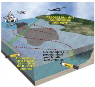
FIGURE 2. An AUV-borne SF/RL sensor detects and geolocates oil beneath Arctic ice, and ARCDEEP enables high-rate data exfiltration while at depth.
