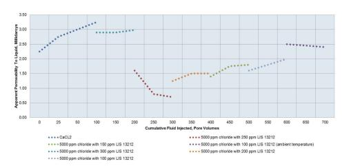
FIGURE 2. This third-party core flow study of field-specific lithology measures the core flow permeability in relation to Clariant's LIS-13212 concentration, using preserved core at field temperature. The 300 ppm LIS-13212 gave the same performance as 30,000 ppm CaCl<sub>2</sub>.
