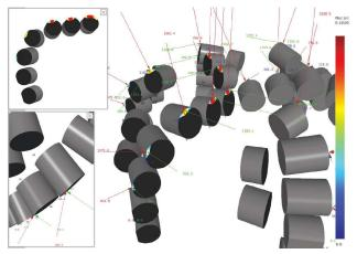
To accelerate the development of rolling PDC cutter technology, the IDEAS drillbit design platform enabled engineers to optimize placement of the rolling cutters on bit blades to ensure reliable cutter rotation. Integration of these cutters was determined by examining the effect different geometric orientations had on three cutter characteristics: durability, appropriate balance of driving force, and aggressiveness. (Image courtesy of Schlumberger)
