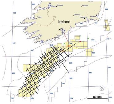
FIGURE 2. The acquisition grid covers the Fastnet basin located in the Irish sector of the Celtic Sea. Most of the program involved simultaneous acquisition of EM and seismic data.
