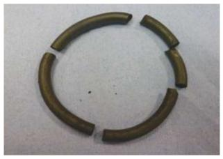
FIGURE 2. This FKM terpolymer is shown after 24 hours in 316°C steam.
