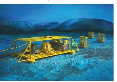
Dependable power supply and distribution will be vital for largescale subsea processing facilities. Siemens' subsea power grid, currently in the detail design and test phase, will include transformers, switchgear, and variable speed drives. (Images courtesy of Siemens)
