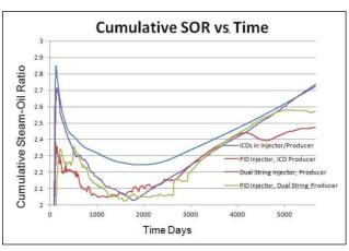
FIGURE 4. The chart compares the cumulative steam-oil ratio for three SAGD well-pair configurations and the base case.
