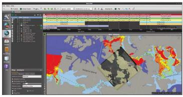
Narwhal can show go and no-go zones based on a particular vessel's ice classification. (Image courtesy of ION Geophysical)
