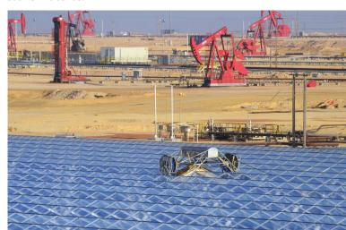
A robot roams the glass rooftops, keeping them clean so the sunshine can be harnessed for solar EOR. Without regular cleanings, the rooftops would be coated in dirt and grime, reducing solar steam output by 3%.
