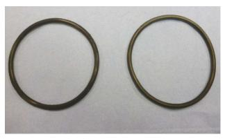
FIGURE 5. Above left: a fresh O-ring seal; Above right: A steamaged EnDura E90SR O-ring seal left in 288°C for 168 hours.
