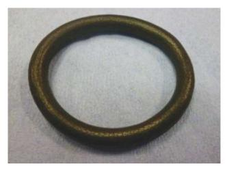
FIGURE 1. Above is a standard EPDM after 24 hours in 316°C steam. Specimen is warped with surface cracking. (Images courtesy of Precision Polymer Engineering)
