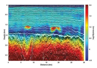
FIGURE 3. A 2.5-D inversion is shown in color as an overlay on a seismic 2-D section. The two fields are seen in yellow and red at a depth of 1.2 km, with Bressay on the left and Bentley on the right.
