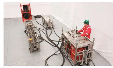
The Flexi-Coil Extended Reach offers an alternative for riser and flowline blockage remediation by using miniaturized coiled tubing principles. (Image courtesy of Paradigm Flow Services)
