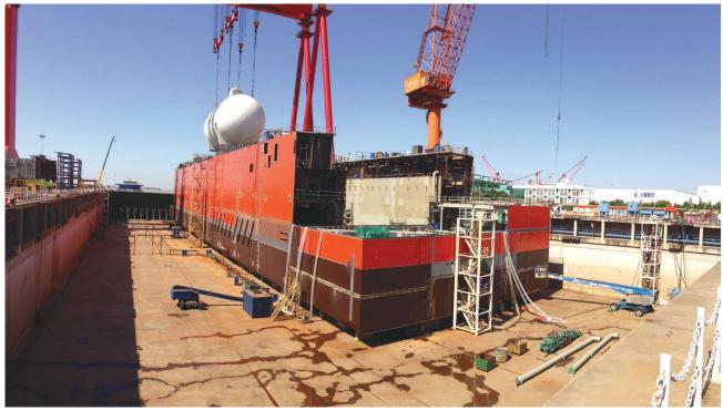
The cargo storage tank is lowered into the hull of the Caribbean FLNG barge at Wison Heavy Industry's shipyard in Nantong, China. (Image courtesy of EXMAR Marine)
