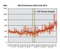
The field in the above graph was under a  $CO_2$  flood and the project was not meeting expectations. With the addition of CESI's **CnF**® foam conformance modifier product, the Operator deemed the project a success after 90 days with an incremental increase of approximately 14,000 barrels of oil at a relative value of less than \$0.60 per barrel... and this increase continued through 150 days.
