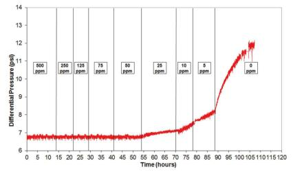
FIGURE 1. This Clariant in-house core flow study shows a client's field-specific lithology, measuring differential pressure in relation to the LIS-13212 concentration using nonpreserved core at an ambient temperature.
