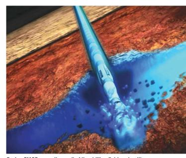
During PMCD operations, all of the drilling fluid and cuttings are lost in the formation. Using statically underbalanced fresh water as drilling fluid in both the drillstring and annulus in PMCD mode minimizes formation damage. (Images courtesy of Weatherford)
