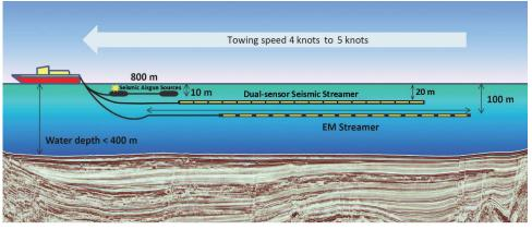
FIGURE 1. This image shows the layout of the EM and seismic acquisition systems. The EM streamer has 72 configurable receiver electrode pairs that are short (about 200 m) at the near offset and long (about 1,100 m) at the far offset. (Images courtesy of PGS)
