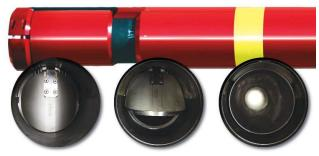
A view down the bore of the DIV shows the flapper transitioning from closed to open position (left to right), facilitating tripping efficiency in both PMCD and CBHP modes.
