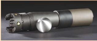
IN-Tallic frac balls seal off the plug for fracturing and then disintegrate in the well to leave an unobstructed ID for production.
