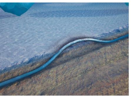
FIGURE 2. Upheaval buckling may expose the pipeline above the seabed.
