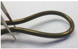
FIGURE 4. This EnDura E90SR O-ring remains flexible without cracking after 24 hours in 316°C steam.
