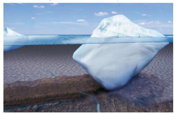
FIGURE 1. Ice keels gouge the seafloor when in water depths shallower than their draft. (Images courtesy of INTECSEA)
