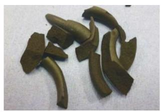
FIGURE 3. This FKM copolymer is shown after 24 hours in 316°C steam.
