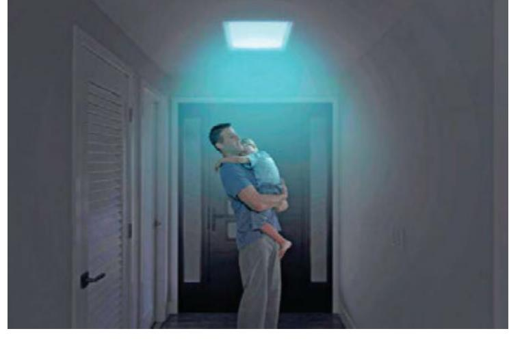
With Solatube Daylighting Systems with Integrated NightLight, you won't have to turn on lights for trips to the bathroom or navigate dark hallways any longer. Solatube Daylighting Systems harvest sunlight on the roof and shoot it down a tube of the most highly reflective material made.
