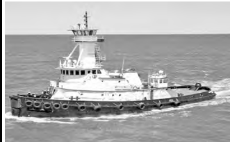
Tug American Patriot: 121' x 34' x 18.8', 4100 BHP, 63 Ton Bollard Pull, ABS Hull & Machinery, A-1 Towing All Oceans, Located GOM. $1.5M
