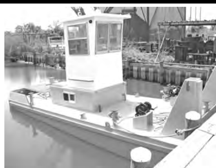
MODEL 2510 25'9" x 10'0" x 4'0" 200 H.P. Single Engine
