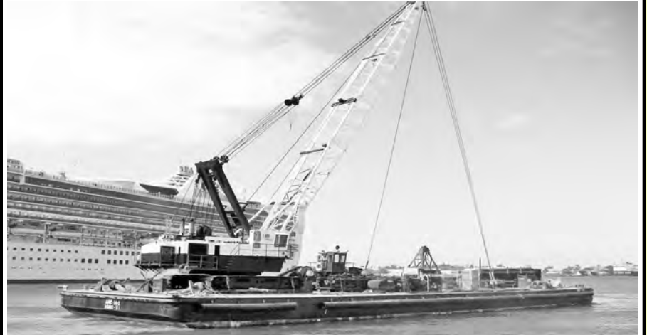
Crane Barge AMC-160: 160' x 51' x 13', 4500 Manitowoc Rated 100 Tons Max Boom Ht 167'; Located Hawaii. $1.5M
