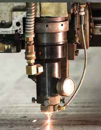
Lasers make quick and accurate complex cuts over and over
