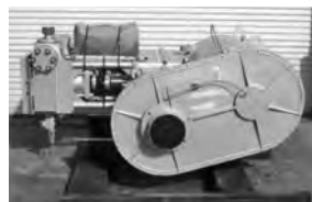
FMCWT2450 Pump 4.5 FLUID END WT2450, Part# P540619, 2400HP, Speed 1950, Gear Ration: 6:39:1 - $110,000
