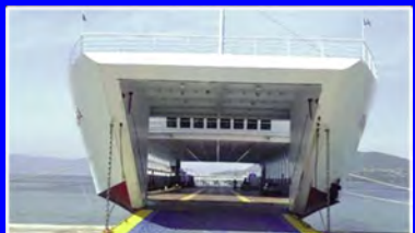
77.6M Ro-Pax Landing Craft 2010 1000 Passenger / 130 Car / 1.8M Draft
