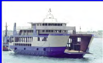
66.75 Ro-Pax Landing Craft 2015 500+ Passenger / 90 Car or 12 Truck
