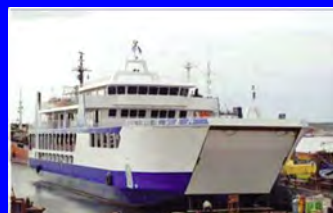
66.75M Ro-Pax Landing Craft 2016 500 Passenger / 90 Car or 12 Truck
