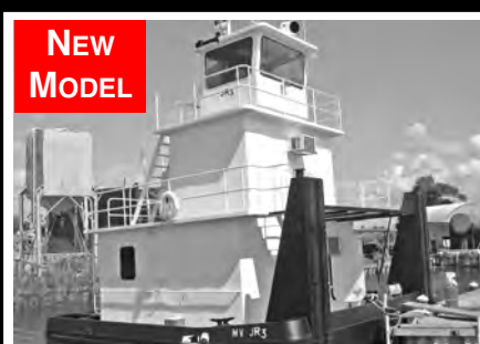
MODEL 2512 25'9" x 12'0" x 4'6" 400 H.P. Twin Engine
