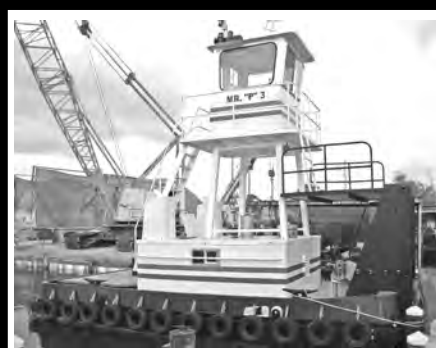
MODEL 2516 25'9" x 16'0" x 5'6" 650-750 H.P. Twin Engine
