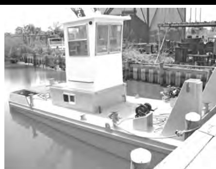
MODEL 2510 25'9" x 10'0" x 4'0" 200 H.P. Single Engine
