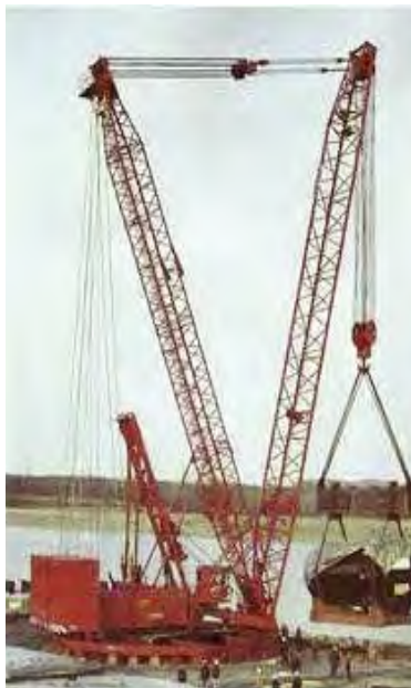
4600 Series 4 Crawler Lift Crane w/ Series 3 Ringer Attachment
