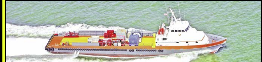
167' WATERJET POWERED USCG T/L ABS CLASS A-1 HSC
