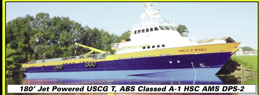
180' Jet Powered USCG T, ABS Classed A-1 HSC AMS DPS-2
