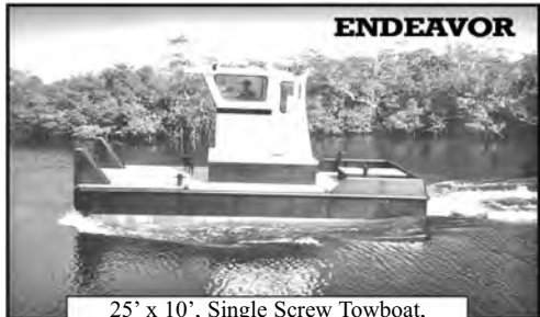
25' x 10', Single Screw Towboat, 225 h.p., Flanking Rudders.
