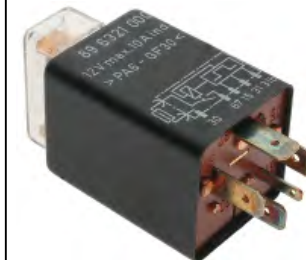
FR100 Fuel Injection Relay 0332204510; 321 906 059C Audi ..... 1980 - 1976 Volkswagen ..... 1984 - 1975
