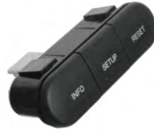
PA996 Information Display Switch 6R3Z-18578AA Ford ..... 2009 - 2006
