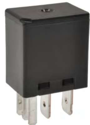
AR7171 Fuel Pump Relay 68055796AA
