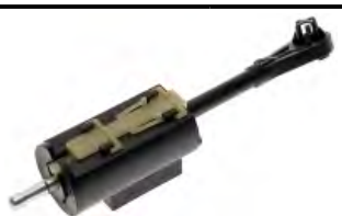
NS5878 Clutch Starter Safety Switch F65Z-7641AA; 1L3Z-11A152AA
