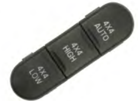
FWD45 Four Wheel Drive Actuator Switch 1L2Z-14B166-AA
