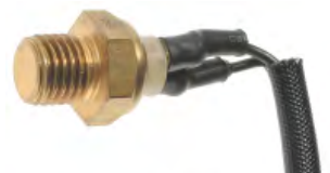
TS5512 Intake Air Temperature Sensor 22630 AA011
