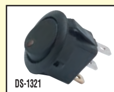
Mini Rocker Switch "ON-OFF" LED illuminated round spot mini rocker switch. 10 Amp., 12 Volt. DS-1321 - Amber DS-1322 - Green DS-1323 - Red
