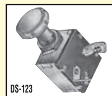
Push Pull Switch Universal 2-position, single pole, single throw. Pull "ON", push "OFF" switch. Furnished with large plastic knob, and 2 screw terminals. Mounting stem dia. 15/32", length 1/2". Rating: 6 Volt 20 Amp., 12 Volt, 10 Amp.
