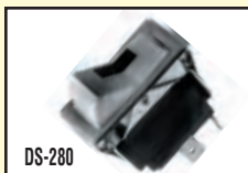
Rocker Switch Universal rocker switch for trucks, buses & recreational vehicles, 35A, 12V silver contact, red illuminated rocker, 2-position "OFF-ON", SPST, 2 spade terminals for circuit. 1 spade terminal for built-in 12V bulb. Black body, white rocker. Kenworth: K-301-1572 OMC: 977743
