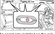
An assist grip installed on the ceiling can be used to support your body while sitting on the seat.
