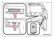
② Press the lock button to lock all the doors. Check that the door is securely locked.
