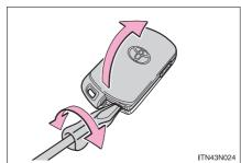
Remove the depleted battery.
