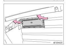
5 Remove the filter and replace it with a new one.
