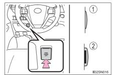
\*: Orange mark on the switch should be visible when the switch is on.
