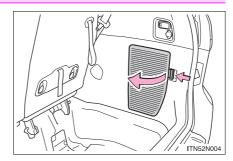
2 Remove the adapter socket.
