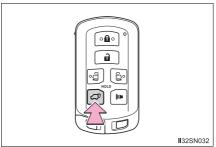
Pressing the switch again while the power back door is operating will cause the operation to reverse. However, the reverse operation cannot be performed for the first second after automatic operation starts, even if the wireless remote control switch is pressed again.
