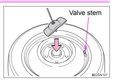
2 Turn the jack handle clockwise to raise the tire until the tire is in the correct position as the jack handle skips.
