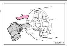
5 Turn clockwise and secure the bulb base.
