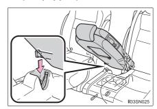
2 Unfold the cushion leg and push down on the seat to engage the front lock.
