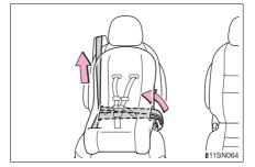
After the shoulder belt has retracted to a point where there is no slack in the belt, pull the belt to check that it cannot be extended.
