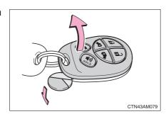
2 Remove the depleted battery.
