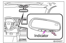
Pressing the button turns the function to off mode. (The indicator also turns off.)
