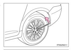
$\fill \fill \fil$ hand until the notch of the jack is in contact with the jack point. The jack point guides are located on the side of rocker moulding. They indicate the jack point posi-
