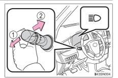
② Pull the lever toward you and release it to flash the high beams once.
