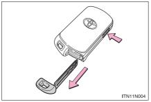
After using the mechanical key, store it in the electronic key. Carry the mechanical key together with the electronic key. If the electronic key battery is depleted or the entry function does not operate properly, you will need the mechanical key.  $(\rightarrow P. 585)$
