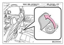
3 Attach the adapter socket over the spare tire clamp bolt.
