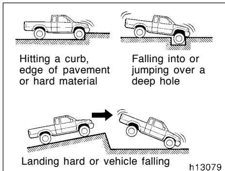
**The SRS airbags may deploy if a serious impact occurs to the underside of your vehicle. Some examples are shown in the illustration.**
