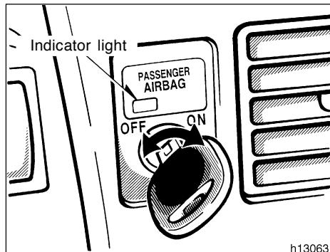
This on-off switch is designed to disable the passenger airbag in order to allow usage, if necessary, of a member of a passenger risk group identified in TABLE 1 is occupying the right front passenger seating position. (For details, see "SRS driver and front passenger airbags" in this section.)
