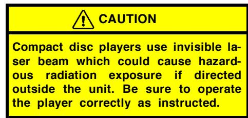
Compact disc players use invisible laser beam which could cause hazardous radiation exposure if directed outside the unit. Be sure to operate the player correctly as instructed.
