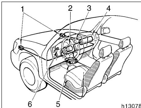
The SRS airbag system consists mainly of the following components, and their locations are shown in the illustration.
