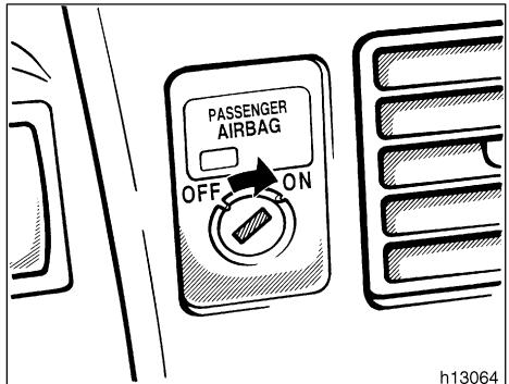
The passenger airbag system is equipped with a manual on-off switch and indicator light. Turning the passenger airbag manual on-off switch clockwise to the "ON" position makes the passenger airbag system operational. Turning the passenger airbag manual on-off switch counterclockwise to the "OFF" position disables the passenger airbag system. The indicator light on the passenger airbag manual on-off switch will come on when the passenger airbag system has been disabled.
