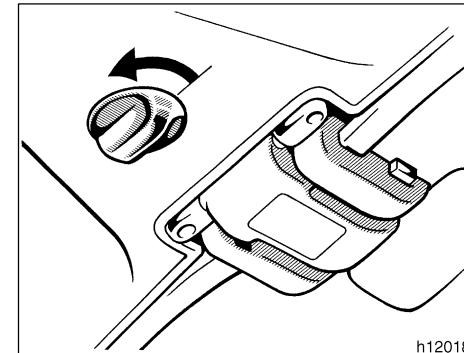
To remove: Support the sun shade panel with your hand while you unlock the sun shade by turning the knob counter-clockwise.
