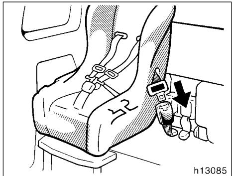
1. Run the lap and shoulder belt through or around the convertible seat following the instructions provided by its manufacturer and insert the tab into the buckle taking care not to twist the belt. Keep the lap portion of the belt tight.
