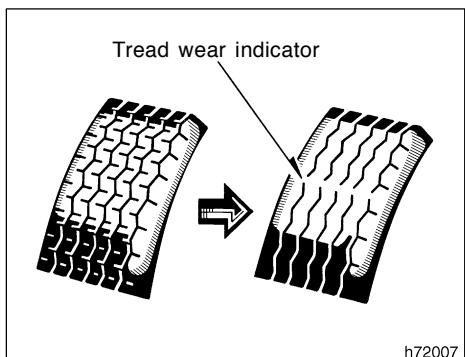
Check the tires regularly for damage such as cuts, splits and cracks. If any damage is found, consult with a technician and have the tire repaired or replaced.
