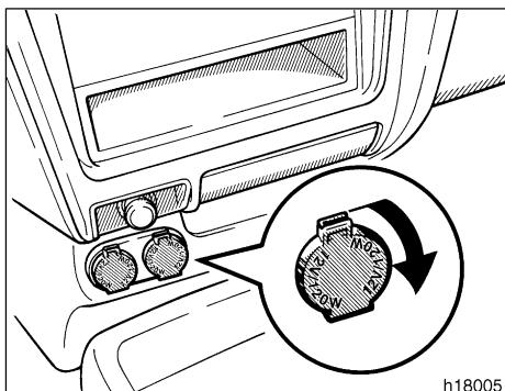
◆ Close the power outlet lids when the power outlets are not in use. Inserting a foreign object other than the appropriate plug that fits the outlet, or allowing any liquid into the outlet may cause electrical failure or short circuits.
