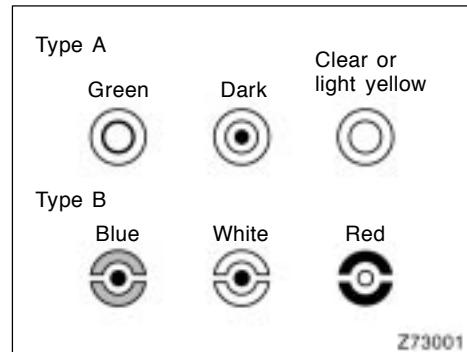
**CHECKING BY HYDROMETER**
