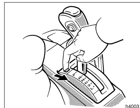
3. Insert the screwdriver or equivalent into the hole to push up the shift lock override button. You can shift out of "P" position only while pushing the button.
