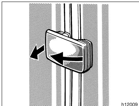
**To unlock the rear window, pull the left end of the latch handle toward you and disengage the right end from the catch.**
