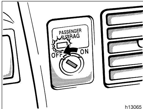
When you put a rear-facing child restraint system which belongs to a passenger risk group on the right front seat, turn the passenger airbag manual on-off switch counterclockwise to the "OFF" position. (For details, see "SRS driver and front passenger airbags" in this section.)
