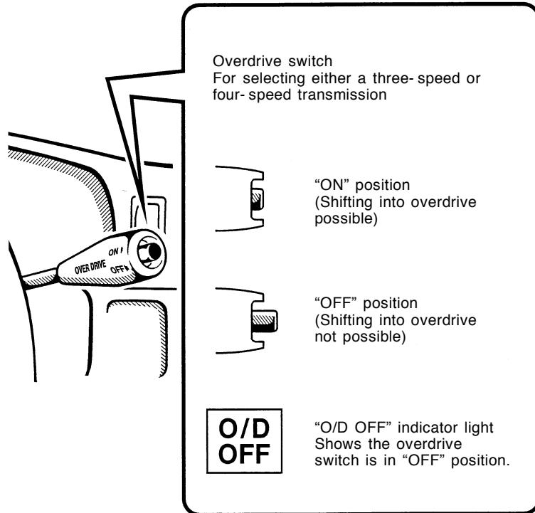
After starting your engine, always turn the overdrive switch on.
