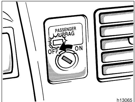
When you put a rear-facing child restraint system on the front seat, turn the passenger airbag manual on-off switch counterclockwise to the "OFF" position. (For details, see "SRS driver and front passenger airbags" in this section.)
