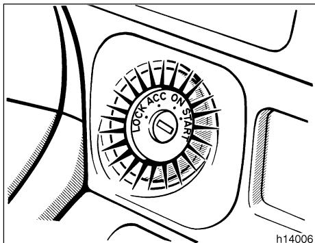
**For easy access to the ignition switch, the ignition switch light comes on when either door is opened.**
