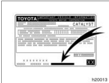
To distinguish your vehicle, refer to the exhaust emission label back of your engine hood. The letter printed on the label as shown means:
