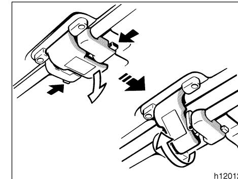
To tilt up the moon roof, first pull down on the handle while pushing in one of the lock buttons. Then push up the moon roof until it locks.
