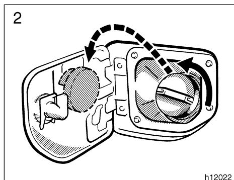
1. To open the fuel filler door, insert the key and turn it counterclockwise. When refueling, turn off the engine.
