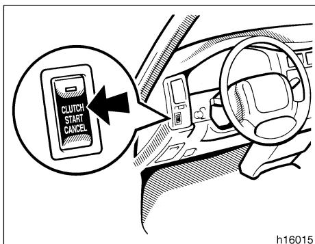
Never use the switch for normal engine starting. Be sure to follow the starting procedure instructed in "How to start the engine" in Section 3.
