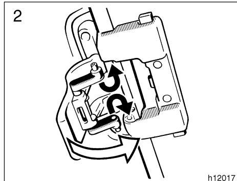
1. Insert the flat hinges of the moon roof panel into the cutouts on the body. Then slowly lower it while holding the roof with your hands.
