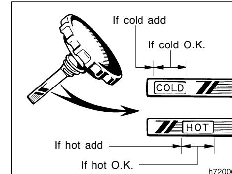
Check the fluid level on the dipstick. If necessary, add automatic transmission fluid DEXRON®II or III.
