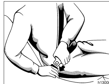
Adjust the seat as needed (front seats only) and sit up straight and well back in the seat. To fasten your belt, pull it out of the retractor and insert the tab into the buckle.
