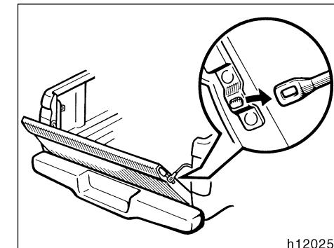
**To lower the tailgate fully, release the support brackets from the lugs as shown.**
