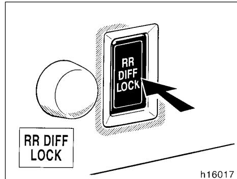
To lock the rear differential, push the switch.
