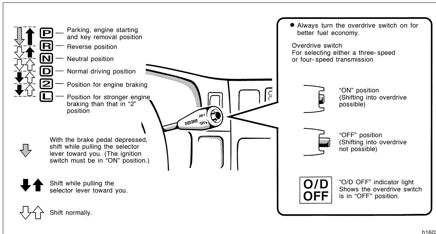
Vehicles with cruise control—When the cruise control is being used, even if you downshift the transmission by turning off the overdrive switch, engine braking will not be applied because the cruise control is not cancelled. For ways to decrease the vehicle speed, see "Cruise control" in this section.
