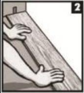
**Figure 2:** Commence installation in the left hand corner. Use shims to allow about 1/4" (6mm) between the plank and the walls, or stationary interior room objects, so that there is room for normal expansion and movement.
