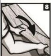
**Figure 8:** Insert the next plank at an angle and snap into place lengthwise. Allow a slight space between the ends and then lock into place by using a tapping block and tap the ends tightly together. The tapping block can be a remnant piece from a cut plank or you can use a block of wood with a routed out interior that does not adversely impact the end side profile.
