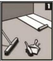
**Figure 1:** Thoroughly clean the subfloor and roll the underlayment as indicated. If installing over concrete a moisture barrier is required (at least 2mm) the plastic film should be overlaid on the adjoining row by about 10" (25cm). When you are applying foam the rows should abut. **Please Note:** (Additional foam is not required if foam is already attached to laminate.)
