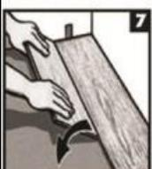
**Figure 7:** Insert the starting piece of plank on the next row at an angle and press forward and down to snap into place.
