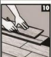
**Figure 10:** To install the last row of the project, place a loose board on top of the last installed plank on the adjoining row. Place another board on top, with the tongue side facing the wall (allow the 1/4" (6mm) expansion joint) and draw a line along the edge of the plank as indicated in the figure and cut along the drawn line. Insert the cut plank against the wall and use a crowbar to ease into position. The shims can then be removed.
