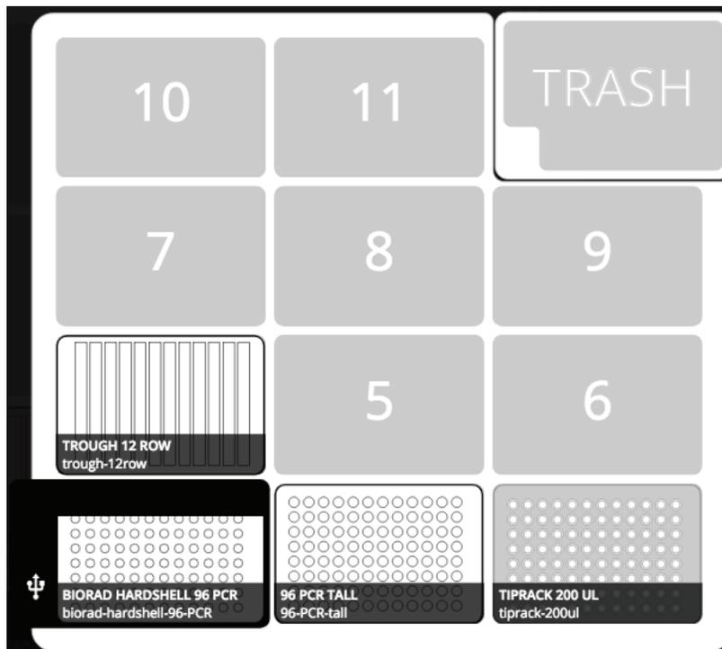
Figure 2. Simple Deck Layout for Nucleic Acid Purification. The Magnetic Module needs to be connected to power source and via USB to the back left of the OT-2. Therefore, we suggest placing the module in the outer slots of the deck to avoid cords interfering with labware on the deck.
