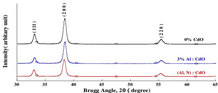
Fig. 1 XRD patterns of undoped, Al doped and (Al, N) dual doped CdO
