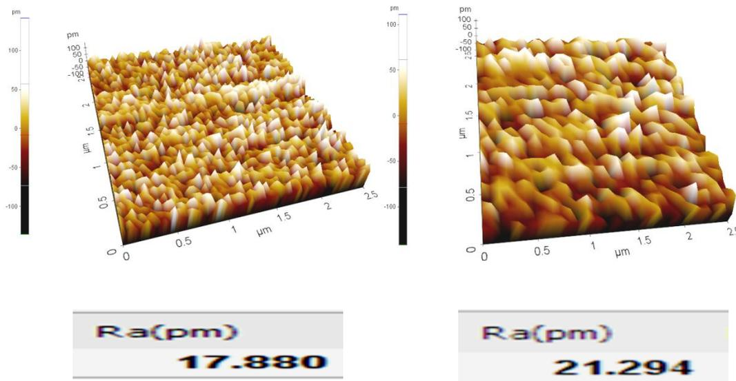
**Fig. 2.** (a-b): AFM images of (a) undoped and (b) 3% Al & 1% N dual doped CdO
