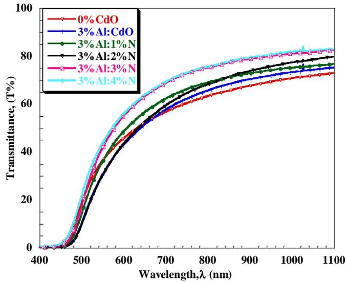
Fig. 3 Optical transmittance spectra of (Al, N) dual doped CdO thin films.
