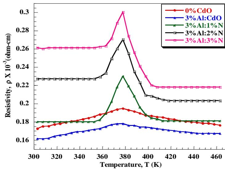
Fig. 5 The plot of resistivity against temperature of CdO thin films
