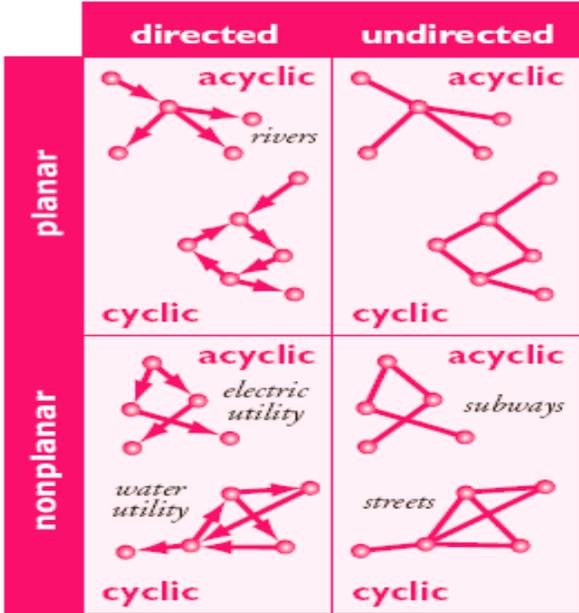
Figure 2: Geometric Network Models
