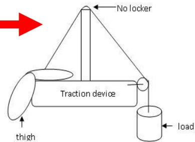
Fig 2.3b Magnification of unsecured rope.
