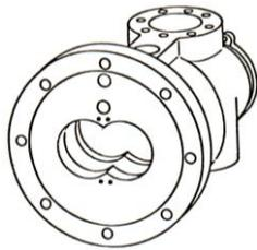
**Rotary Twin Screw Casing**
