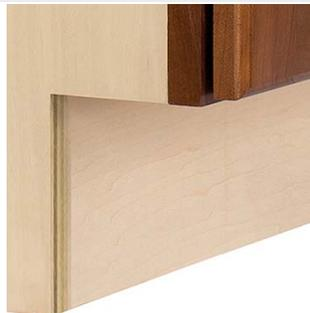
4 1/2"H x 3 3/8"D Toe Kick cut out, 1/2" unfinished plywood toe kick extends to cabinet floor for captive construction
