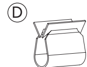
ARTOCLIP Retaining clip 1/2 x 7/16 x 1/4" (12,7 mm x 11,1 mm x 6,35 mm)
