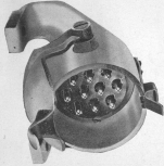
Plate No. 12-A. 1/2 Size TRAIN LINE JUMPER PLUG AND SOCKET, SUBWAY DIV.
