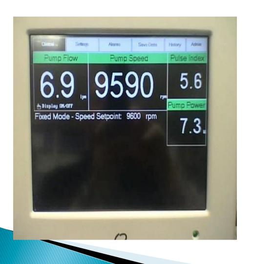
Pump Speed (RPM) – How quickly the pump rotates
