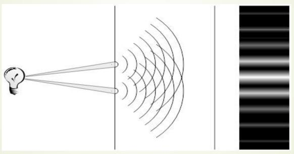
Two slits without photon detectors; result - alternating bands of light and dark
