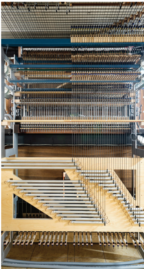
Key and coupler action behind console. Carbon fiber trackers enable a light and secure action.
