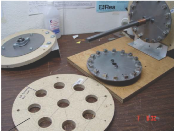
1/2" wood, for holding generator coils
