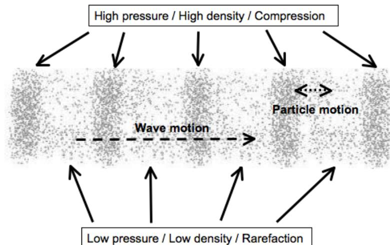
When regarding sound waves in this way, you can see that the behavior of the air particles is very like the behavior of the coils on a long spring that become stretched and compressed as a longitudinal wave moves along it.
