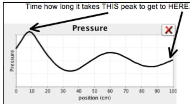
Repeat this measure for different settings of the 'Frequency' slider control, but do not set it very high or it will be difficult to follow a particular peak. *(Remember, you are looking at how fast a peak in the pressure wave moves from left to right, not how fast the graph goes up and down at one particular location.)*
