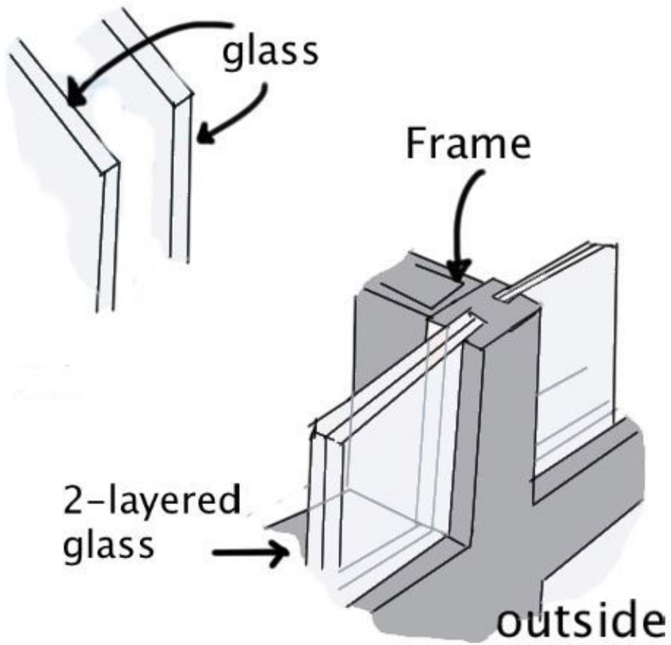
*Figure A2: A closer look at the frames and insertion of the glass*
