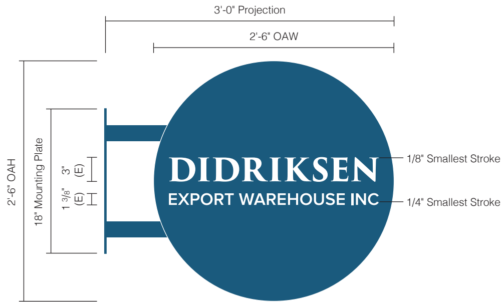
A Sign Elevation - Front View - Side A Scale: 1"=1'-0"
