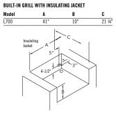
Note: Insulating jacket required for all grills installed into a combustible enclosure. For natural gas grills,
