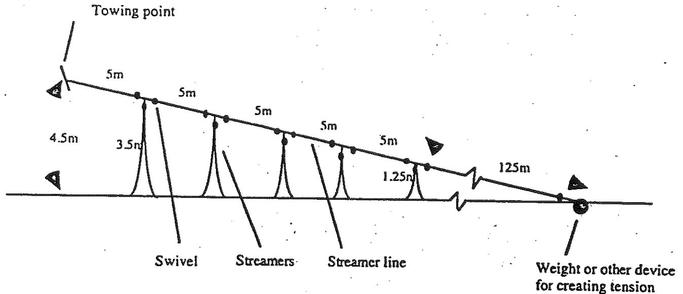
Figure 2 to Part 380—The Use of Streamer Lines to Minimize the Incidental Mortality of Seabirds in the Course of Longline Fishing or Longline Fishing Research Operations in the Convention Area (see § 380.27 for specifications on use)
