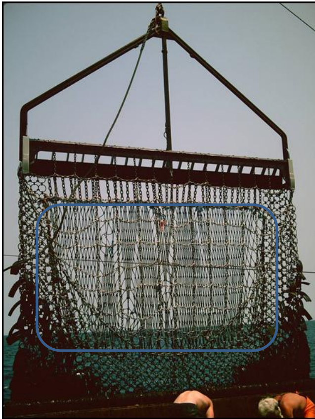
Figure 4. Turtle Chain Mat Example. The chain mat is the rectangular grid of chains in the center of the dredge (outlined by the blue box) that keeps turtles from swimming into or being caught in the dredge bag.
