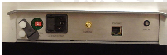
Cover open allowing access to calibration switch
