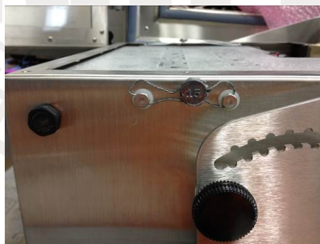
Outside seal holds internal sealing plate in place
