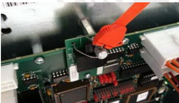
Figure 1. Wire Security Sealing Provision
