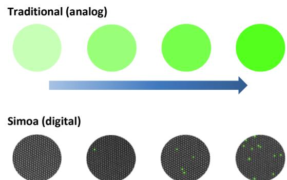
**Figure 1.** Top, Analog measurements give increasing intensity as the concentration increases. Bottom, In contrast, digital measurements are independent of intensity and simply rely on a signal/no signal readout.
