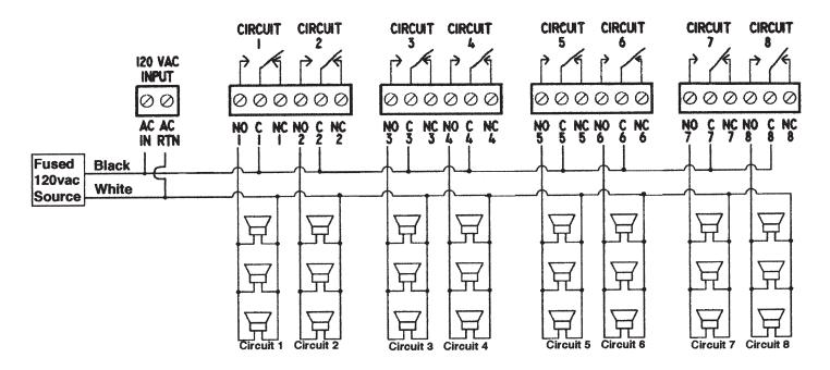
This diagram is using 120vac bells (user supplied step-down transformer required for low voltage (24vac) signals).
