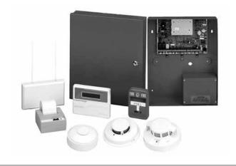
Designed to integrate seamlessly with CCTV, access control and a full range of fire and burglary components, Honeywell's VISTA-32FB provides the ultimate protection of life and property. The UL listed Commercial Fire and Burglary Control Platform can control up to two separate partitions independently, and supports up to 32 zones/points using hardwired, wireless and addressable V-Plex technologies.
