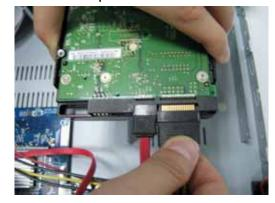
**Step4** Put the HDD to the DVR, and have the SATA HDD fixed in the DVR.
