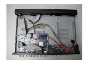
**Step3** Get a compatible SATA HDD, and connect it to the power connector and data bus connector.
