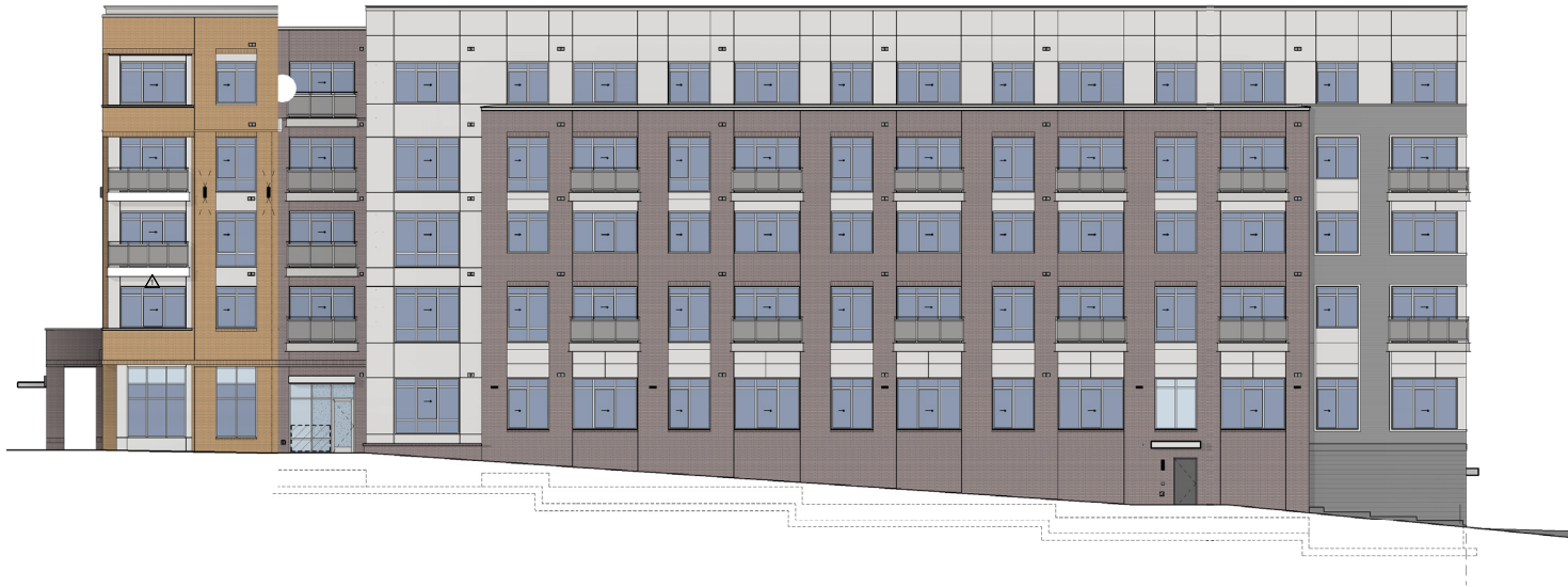
2 EAST BUILDING ELEVATION - SOUTH D 1/8" = 1'-0"
