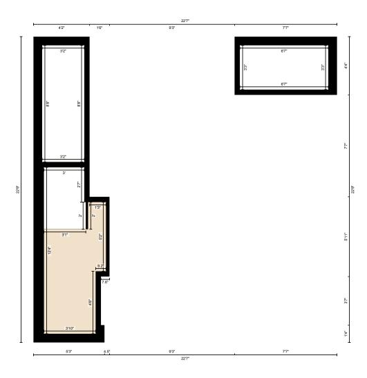
Measurement Diagram for: 2nd Floor Exterior Wall Thickness: 7.8 in
